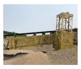
Built a portable truss section with a gravity take up system in the truss with a sliding track system for the take up pulley to slide on, eliminating the vertical gravity take up pulley and lowering the height of the conveyor. This allowed the mesh guarding to be attached to the truss section and move the gravity weight system to the side of the conveyor truss where it can be completely guarded.
