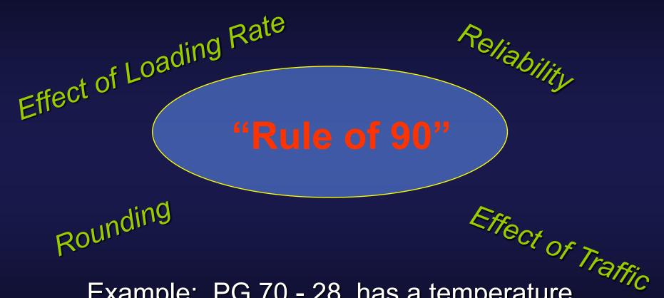
Example: PG 70 - 28 has a temperature range of 70 to - 28 or 98 C. Therefore, this binder is probably modified !! (Depends on Asphalt Source!)
