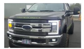
Companies can utilize after-market programmable flasher systems that are designed to strobe flash exterior lights. This system allows smaller vehicles to have a higher degree of visibility to surrounding heavy equipment.
