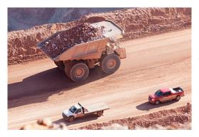
Standard work vehicles are smaller than heavy equipment and can potentially be difficult to see by the larger heavy equipment. This hazard could lead to equipment damage, safety stand-downs, lost time, worker injury, and/or death.
