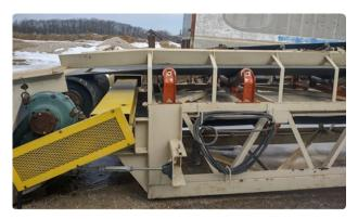
Portable conveyor systems without walkways are difficult to provide proper fall protection systems. When maintenance is required, to effectively reach the area, miners must climb onto the belt which can create a hazard of falling.
