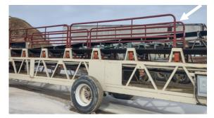
Added portable handrail/cattle gates that can be easily removed to the sides of the conveyor system. This provides a safe working platform when performing maintenance and working on top of the conveyor belt.
